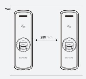
Install BioEntry R2 onto the fixed bracket.
