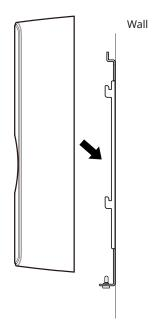
Connect BioEntry R2 to the bracket by rotating the product fixing screw.
